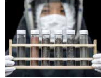
Metals that can be collected with LIB recycling, such as black mass
